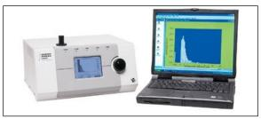
**Figure 4.** TSI Aerodynamic Particle Sizer (APS) model 3321 used to measure total particle concentration and particle size distribution of the challenge bioaerosol. Range  $0.54-20.0 \ \mu m$  aerodynamic diameter, with 1 particle/L detection limits.
