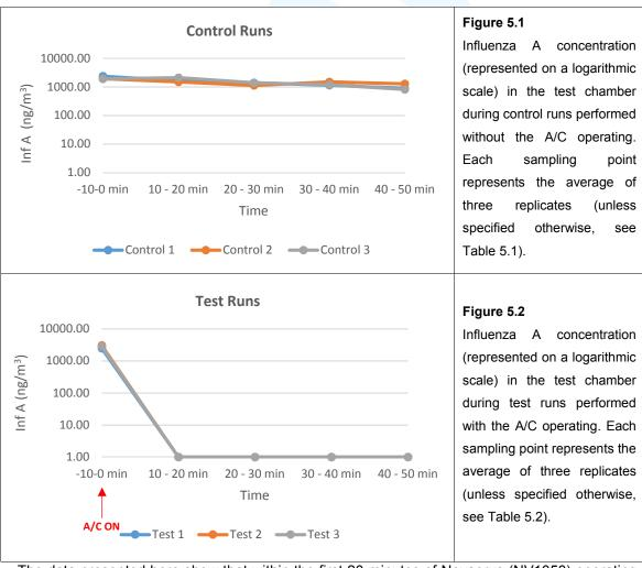
The data presented here show that within the first 20 minutes of Novaerus (NV1050) operating at max speed, the Influenza A concentration in the test chamber was reduced to less than the limit of detection of the assay (<0.156 ng/ml).
