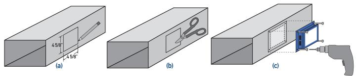
FIGURE 1 - Mounting on duct
